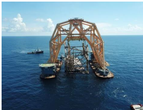
VB-10000 USING ONE CLAW TO LIFT SUBMERGED TANK WEIGHING 1,500 TONS – NO DIVERS NEEDED
