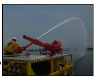
THE TT-750 IS QUICK TO SET UP AND WHEN USED IN COMBINATION WITH THE SUPPLIED BOOSTER UNIT, CAN BE PLACED ON THE DECK OF A LARGE VESSEL WITH NO LOSS OF CAPACITY.
