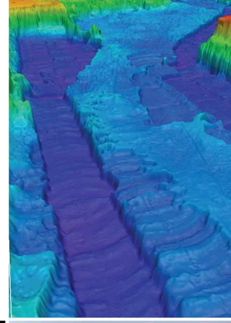
Above right: Multibeam image of dredged channel. Bottom right: USCGC Healy in Northern latitudes. Below left: Multibeam image.
