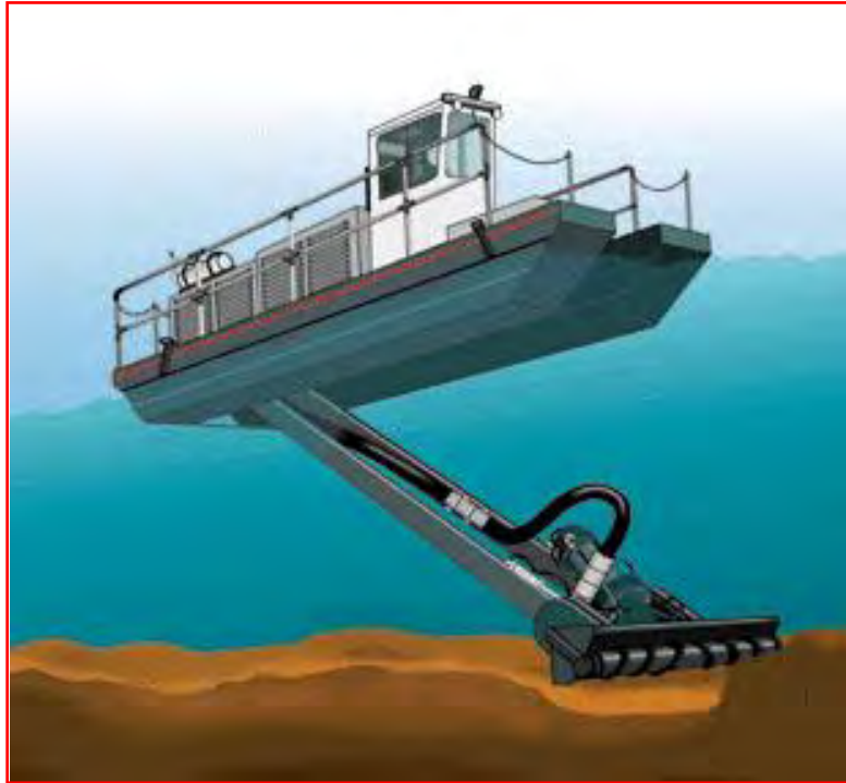
T&T's Submerged Oil Rotary Dredging System
